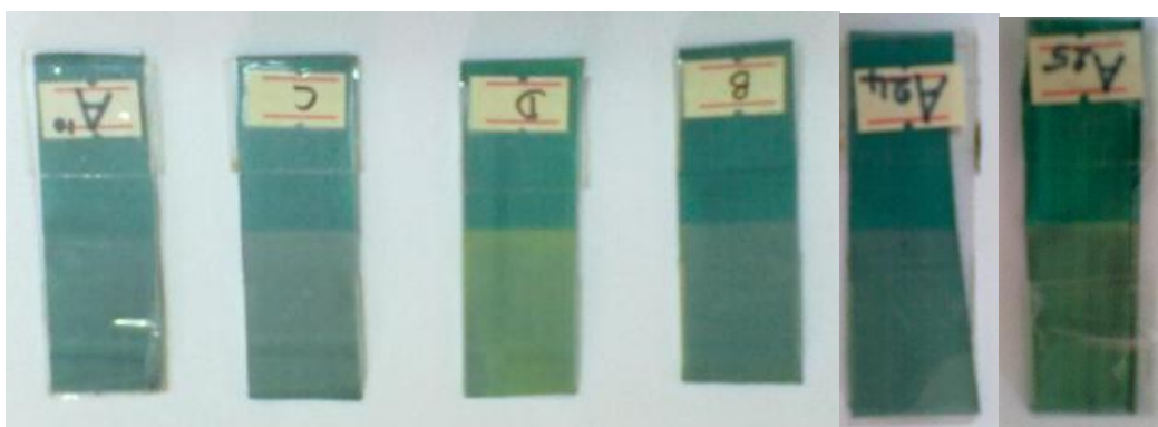
Fig 6: Dyed without bleaching (B), dyed with bleaching (A 24 ), dyed with naphthalene (A 10 ), dyed with NaCl (C), dyed with Na 2 CO 3 (D) and dyed with bleaching and Naphthalene (A 25 ).
